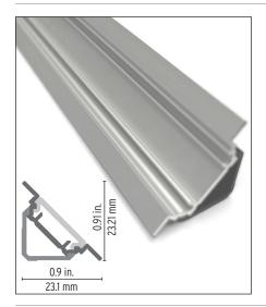
Contour 1907 is a corner profile that offers a minimum of mounting height which should be used in combination with our high density (HD) LED tapes. It can be used as undercabinet lighting, corner lighting or furniture lighting. It can be equipped with a huge variety of different diffuser optics (semi-opal and opal). The channels and optics are field cuttable and provide heat sink for LED tapes up to 7.6 W/ft. Silver, White or Black
