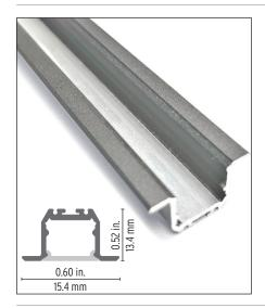
Contour 1512 has been designed for recessed applications with small spaces. With its height of 0.52" (13.4 mm) it fits perfect into dry construction. It has an opal cover and a diffused light output surface. The channels and optics are field cuttable and provide heat sink for LED tapes up to 7.4 W/ft. White or black finish.
