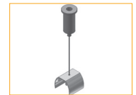
Pendant Mounting Kit 13000161, Silver 13000161-SCH, Black 6.5 ft cable length, recommended spacing is 3.25 ft.
