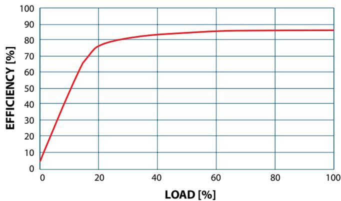
277VAC INPUT EFFICIENCY VS. LOAD
