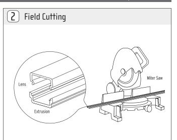
Cut extrusion and lens to the desired length in the field. For short runs (<78"), cut all parts to the same length by using the proper blades for aluminum/plastic cut.
