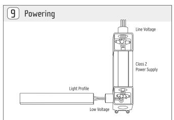
Ensure the correct (wattage & voltage) power supply is used to power the tape. For more information please refer to power supply and LED tape wiring instructions.
