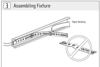
Attach the quick connector or solder lead wires to one side of the tape. Shorten the LED tape to desired length by cutting along the marked area in between the solder pads. Remove paper backing from the adhesive tape firmly press down onto the aluminum surface. Uncoil and peel minimal amount as you install to avoid collection of debris. Excessive uncoiling and peeling of tape create ripples and air bubbles on the tape that should be avoided.
