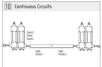
Maximum run length of the tape depends on the power supply specifications. For continuous runs, place the power supplies either at both ends of the run or in the middle of the run next to each other.
