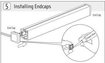
Feed the lead wires through or behind the endcap. Add Super Glue inside and around end cap to secure it in place. For select models, use torque bit to screw the endcap. If applicable, secure the Quick Connector by adding super glue and pressing it onto the extrusion.
