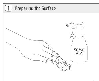
Thoroughly clean the area where tape lights will be installed. Using a 50/50 alcohol mix, clean the area where LEDs will be applied and allow time for alcohol to dry for 5 minutes.
