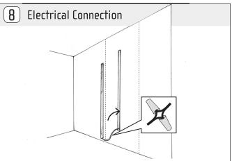
Use plenum rated low voltage connectors (by others) to make the electrical connection between the driver and the light profile. Feed the extra wires and connectors through the opening of the mounting profile.
