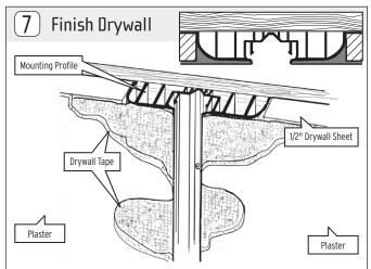
Cover over the sides of the mounting profile by using drywall tape and plaster. Finish the drywall installation with paint.
