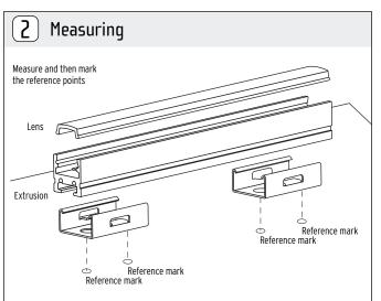
Align the mounting channel to the determined location. Mark reference points to install to the surface. The location of the power supply or wiring box should be determined prior to installation.
