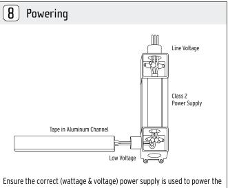
Ensure the correct (wattage & voltage) power supply is used to power the tape. Then proceed to connect low voltage wires from extrusion to power supply. For more information please refer to power supply and LED tape wiring instructions.
