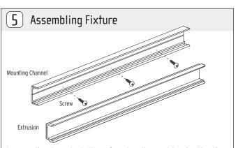
Lay mounting channel onto the surface along the pre-determined locations and secure using the screws provided by others. Using the mounting bracket is necessary for relevant models (0002, 0005, 0013, 0016, 0022). Gluing the channel to surface without using the mounting bracket should be avoided. Snap the channel into the mounting channel. Offset them for longer runs.
