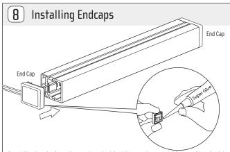
Feed the lead wires through or behind the endcap. Add Super Glue inside and around end cap to secure it in place. For select models, use torque bit to screw the endcap. If applicable, secure the Quick Connector by adding super glue and pressing it onto the extrusion.
