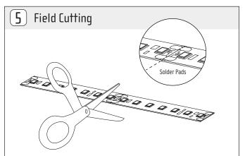
The tape can be cut with a pair of scissors at marked locations in between solder pads. Refer to the product datasheet for exact cut lengths. Always cut from end with no connector/wire leads. Then use either soldering or Quick Connect methods to power cut sections.
