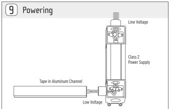
Ensure the correct (wattage & voltage) power supply is used to power the tape. Then proceed to connect low voltage wires from extrusion to power supply. For more information please refer to power supply and LED tape wiring instructions.
