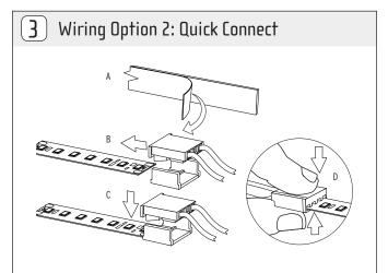
The tape can be connected to Quick Connect terminals supplied by LED Linear. Peel the backing of the tape about half inches (A). Carefully slide the LED tape into the connector (B). Make sure that the polarity is correct: red(+) and black (-). After making sure that the contacts overlap (C), crimp the connectors by pressing tightly (D).
