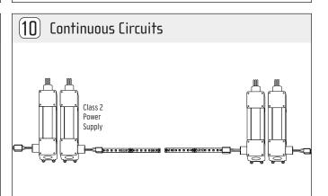
Maximum run length of the tape depends on the power supply specifications. For continuous runs, place the power supplies either at both ends of the run or in the middle of the run next to each other.
