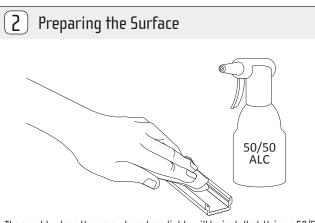
Thoroughly clean the area where tape lights will be installed. Using a 50/50 alcohol mix, clean the area where LEDs will be applied and allow time for alcohol to dry for 5 minutes.
