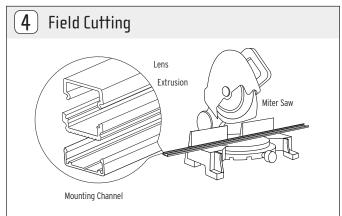
Cut extrusion, lens, & mounting channel to the desired length in the field. For short runs (<78"), cut all parts to the same length by using the proper blades for aluminum/plastic cut. For longer runs it is recommended to cut the mounting channel longer than the extrusion to accommodate end to end connections.
