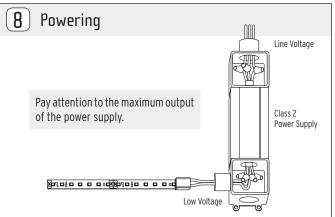
Connect positive wire to RED (white) low voltage wire from power supply. Also, connect negative wires to BLACK (gray) low voltage wire from power supply. Refer to the power supply data sheets for the maximum cable length from power supply to the product.
