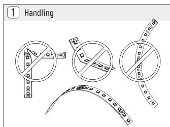
Mechanical stress of the tape must absolutely be avoided. Assembly must not lead to damage or interruption of the circuit paths. Avoid Electrostatic Discharge with proper equipment. Do not attempt to bend the tape horizontally or with sharp edges. The recommended minimum bending radius is 1".
