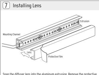
Snap the diffuser lens into the aluminum extrusion. Remove the protective film from the diffuser lens.
