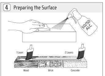
Wipe the surface with 50/50 alcohol solution to provide a clean mounting surface, free of oils, silicones and dirt particles. The mounting surface must have be smooth and have sufficient structural integrity. For porous materials like wood, brick or concrete, optional painting/priming the surface increases bonding power.
