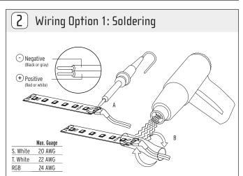
Lead wires can be soldered onto the tape. Solder connections should only be performed manually on designated solder pads that are marked as "24 V"(A). The maximum solder time is 3 seconds and the maximum soldering temperature is 662°F (350°C). After soldering, use shrink tube (provided by others) over the connection and cure with heat gun (B).
