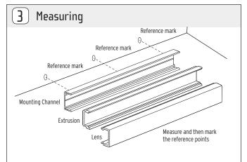
Align the mounting channel to the determined location. Mark reference points to install to the surface. The location of the power supply or wiring box should be determined prior to installation.
