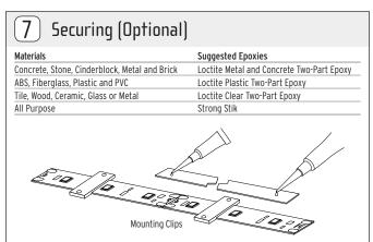
For additional security, use mounting clips every 12" (supplied by others) or apply small amounts of epoxy at each end to increase holding force. Refer to table for recommended epoxy brands. Avoid installing the tape overhead without taking additional securing measures.
